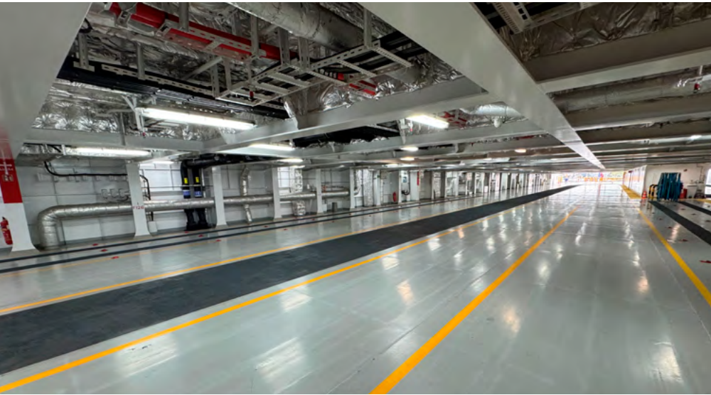
Upper car deck with special non slip walk way for bicycles and motorbikes
